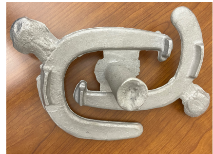
Example of an incomplete casting of horseshoes. This is caused by a low-temperature pour.
